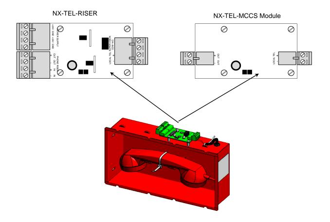
Figure 52 – NX-TEL or NX-TEL-MCCS Command Center Firefighter Phone and Enclosure
