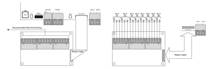
Figure 63 – NX-EM-RL8 Installation and Wiring
