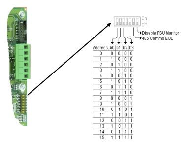
Figure 58 – Switch LED Module Addressing
