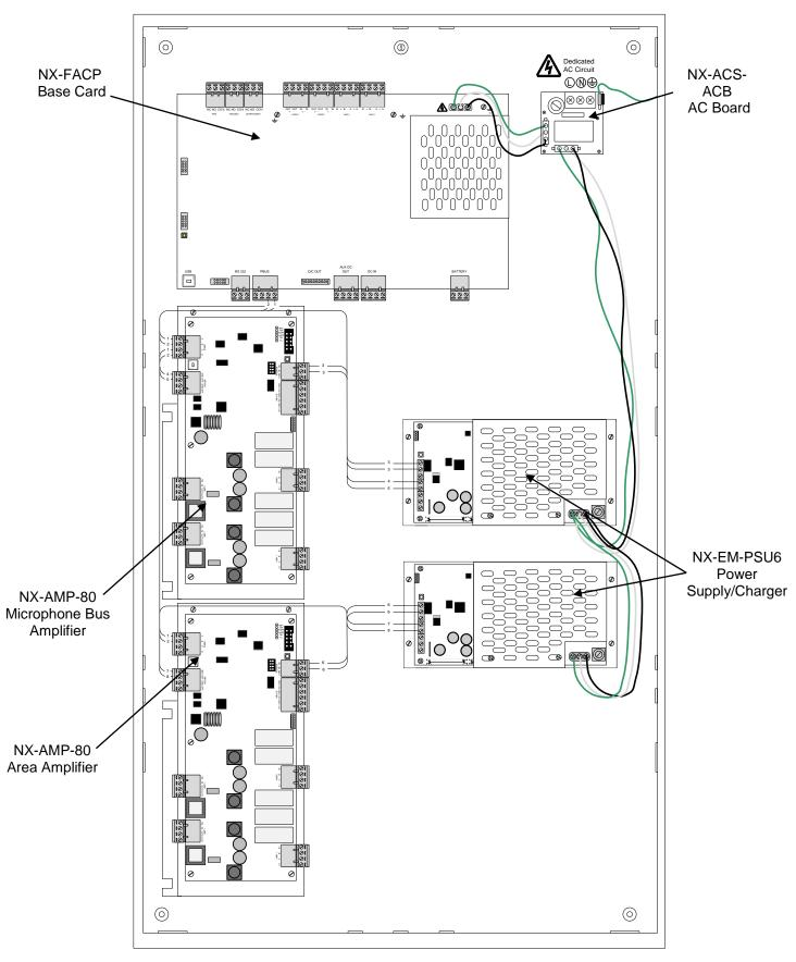
Figure 2 – NX-CC02-BB-BB Back box (Configured with NX-FACP, One Microphone Bus Amplifier and One Area Amplifier)
