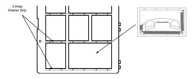
Figure 55– NX-TEL2-MCCS (/P) Firefighter Phone System2 Phone Enclosure Installation
