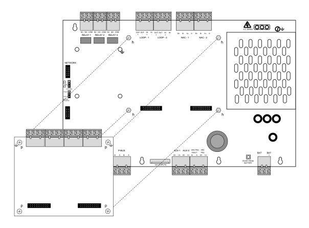
Figure 39 - NX-EM-LPD or NX-EM-NAC Module Mounting to NX-ACS-2L
