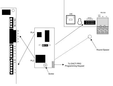
Figure 42 - NX-SEB Installation and Wiring
