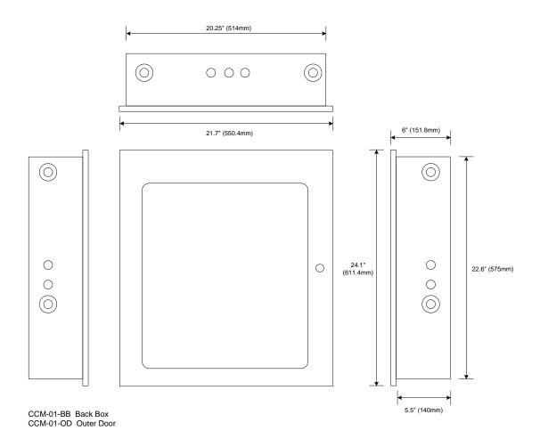
Figure 3 - NX-CC[x]-16 and NX-CC01 Enclosure Dimensions
