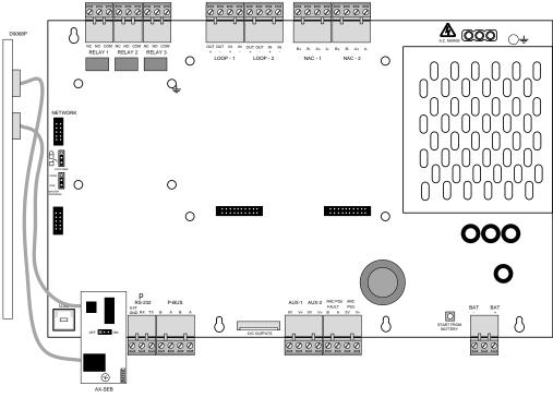
Figure 41 - D9068P Installation
