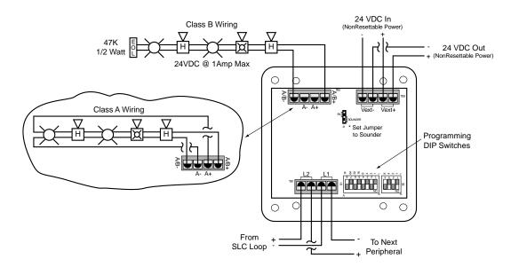
Figure 18 - S-A4046 Notification Appliance Circuit Wiring
