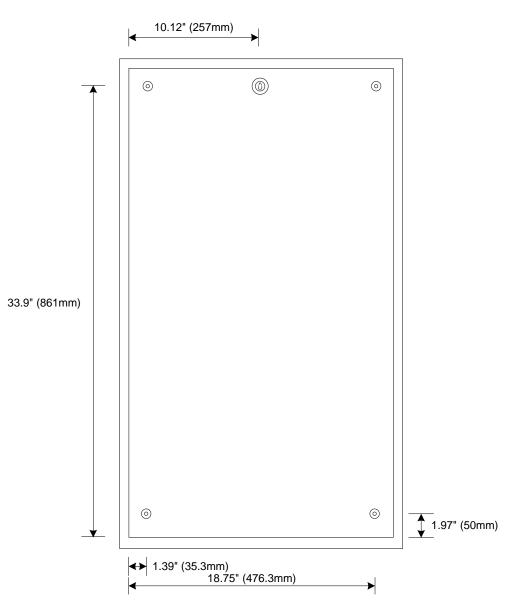
Figure 4a - NX-CC02-BB-BB Mounting Dimensions
