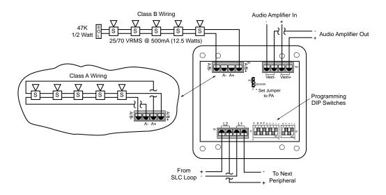
Figure 19 - S-A4046 Speaker Circuit Wiring
