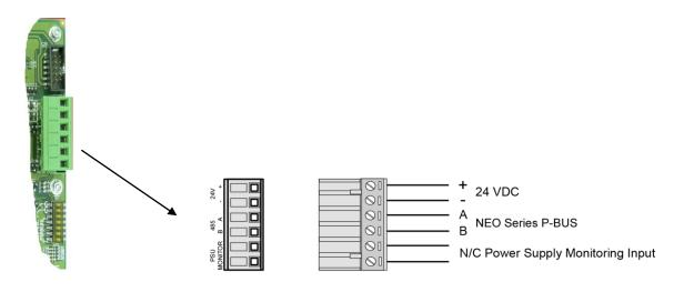
Figure 59 – Switch LED Module Wiring
