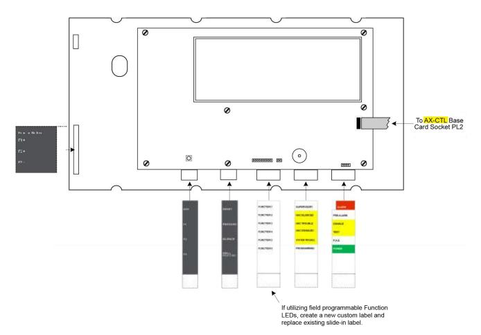
Figure 23 – Slide-in NX-ACS-DSP Labels
