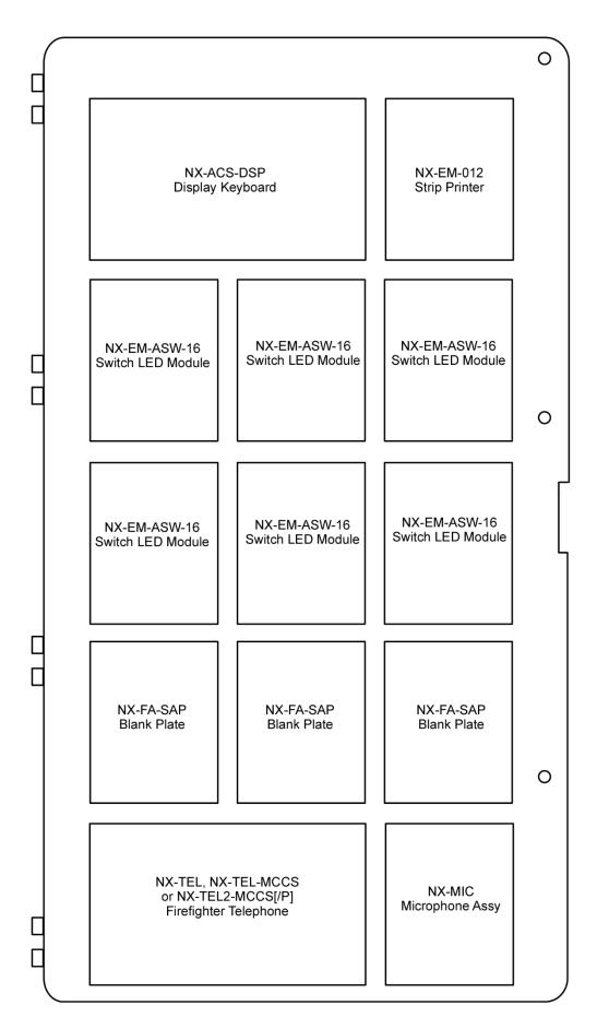
Figure 2a – NX-CC02-BB-ID2 Inner Door Shown with Option Modules
