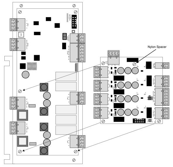
Figure 34 – NX-ZS to NX-AMP-80 Mounting
