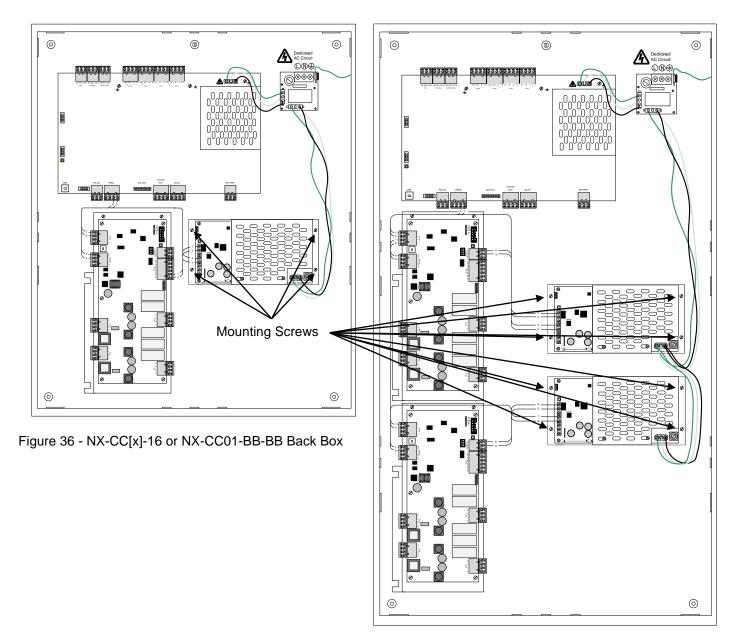
Figure 37 - NX-CC02-BB-BB Back Box w/two (2) NX-AMP-80s
