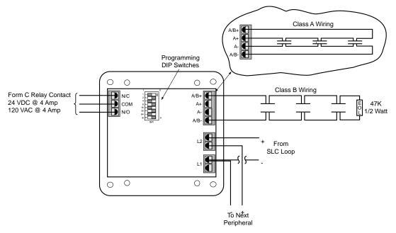
Figure 17 - S-A4049 Wiring
