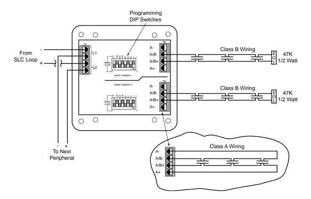
Figure 15 - S-A4042 Wiring
