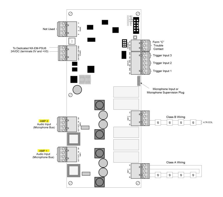
Figure 31 - Hardwired NX-AMP-80 Amplifier
