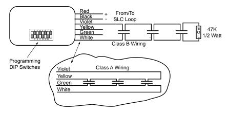
Figure 13 - S-A4048 and S-A4047 Wiring
