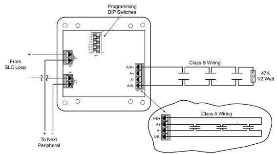
Figure 14 - S-A4043 and S-A4044 Wiring
