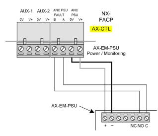
Figure 62 – NX-EM-PSU Expansion Power Supply Wiring
