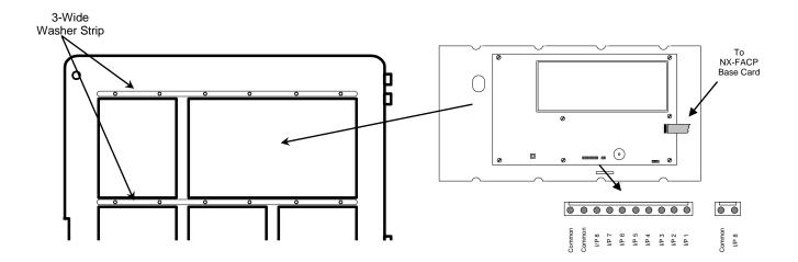
Figure 24 - NX-ACS-DSP Installation and Inputs
