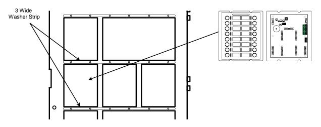
Figure 57 – Switch LED Module Installation
