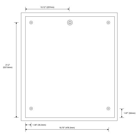
Figure 3a - NX-CC01-BB Mounting Dimensions
