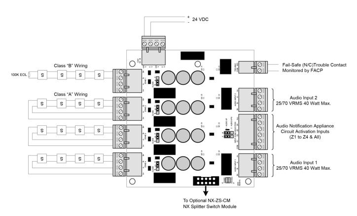
Figure 35 – Optional NX-ZS Audio Zone Splitter Module
