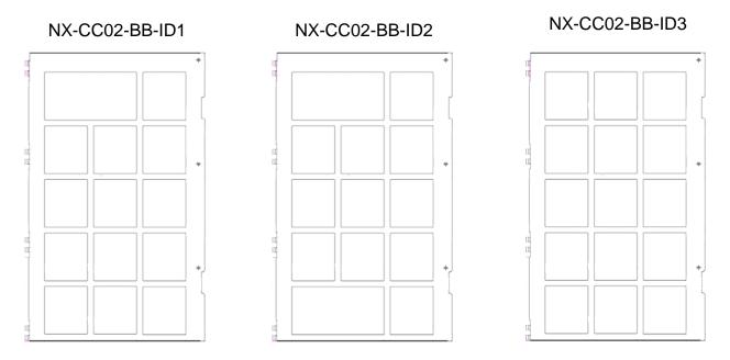
Figure 6 – NX-CC02-BB Modular Command Center Inner Doors
