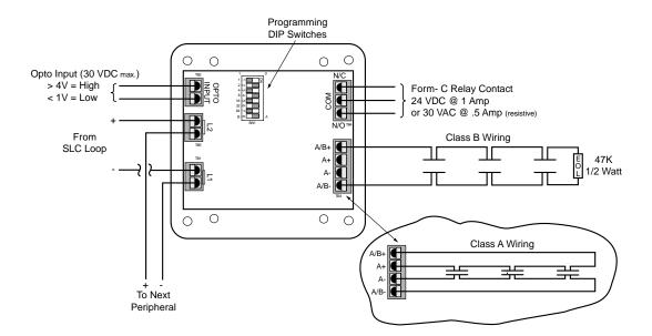
Figure 16 - S-A4045 Wiring
