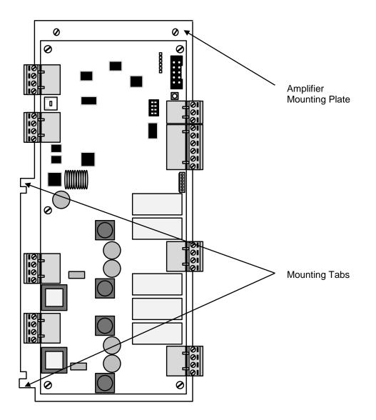
Figure 33 - NX-AMP-80 Amplifier Replacement
