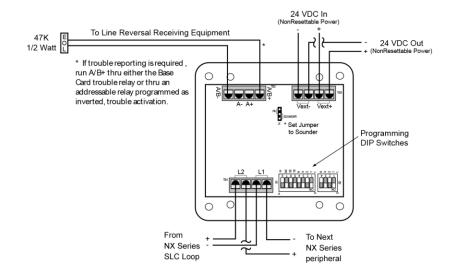
Figure 46 - Reverse Polarity Wiring
