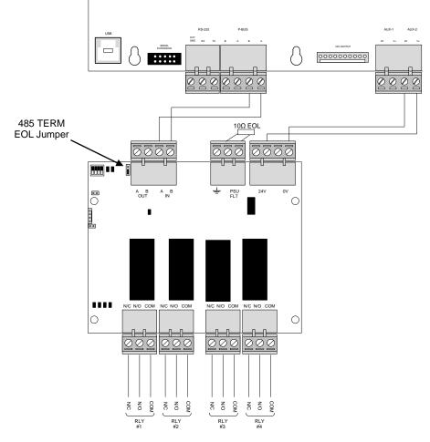
Figure 64 – NX-EM-RL4 Installation and Wiring
