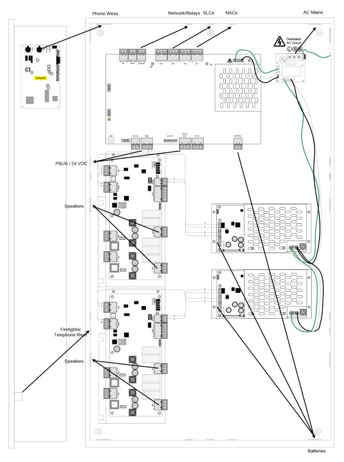
Figure 69 - NX-CC02-BB Modular Command Center Wire Routing
