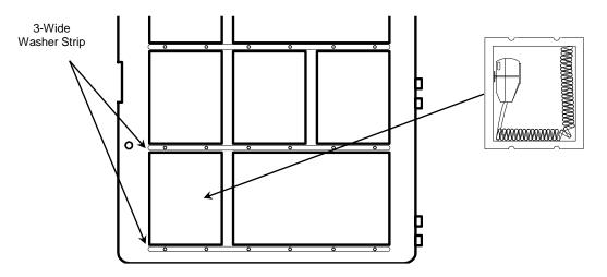
Figure 49 - NX-MIC, Microphone Assembly
