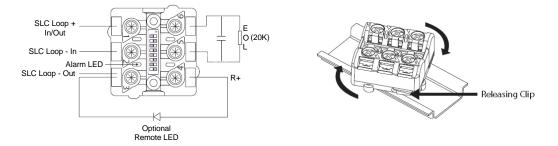
Figure 12 - S-A4041 Wiring & Optional Mounting
