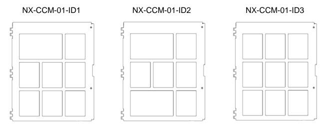
Figure 5 – NX CCM-01 Modular Command Center Inner Doors
