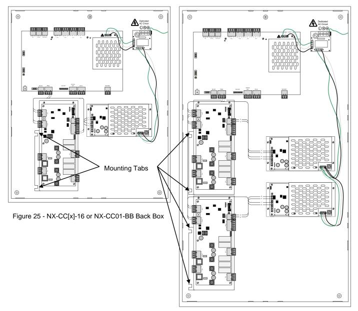
Figure 26 - NX-CC02-BB-BB Back Box w/two (2) NX-AMP-80s
