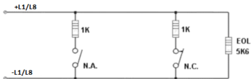
Standard connection diagram of NO/NC contacts
