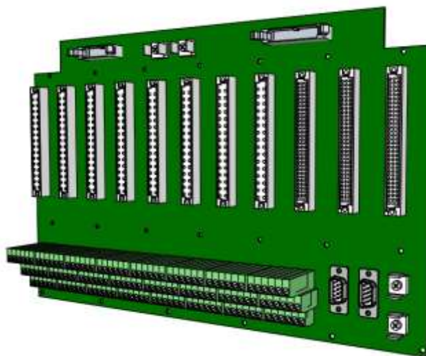
I/O rack SI-2204-1 PCB view
