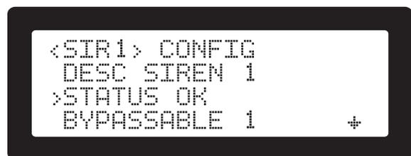
Figure 35. Bypass through STATUS screen
