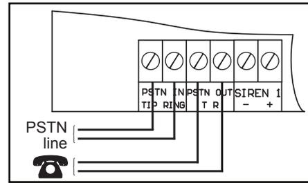
Figure 65. System required phone line connection
