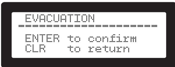
Figure 53. Set global evacuation from keypad screen
