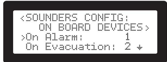
Figure 63. On-board devices configuration screen
