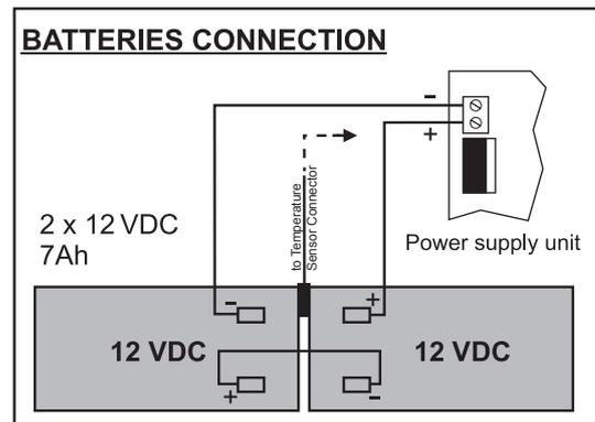
Figure 5. Battery installation
