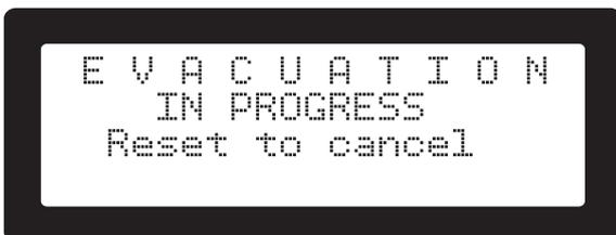
Figure 54. Set global evacuation from keypad screen
