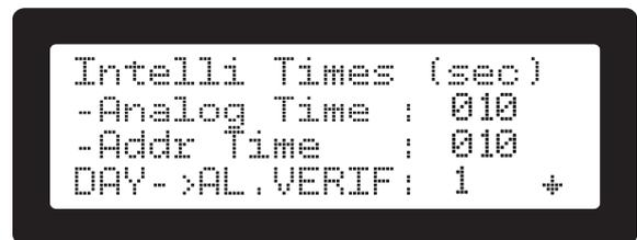
Figure 41. Day/Night, Alarm Verification first screen
