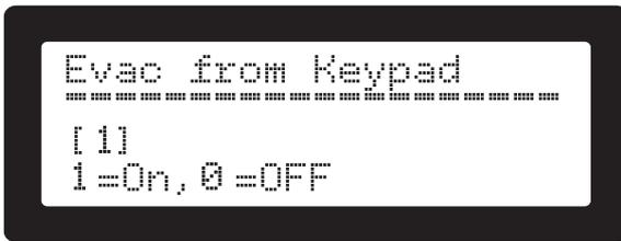
Figure 62. Evacuation from Keypad activation screen
