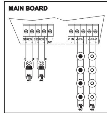
Figure 38. Analog input and output zones termination
