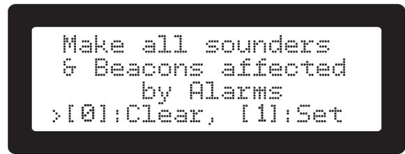
Figure 61. Sounders alarm group configuration screen
