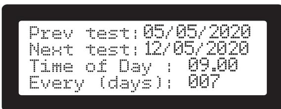
Figure 48. Set Periodic Test screen
