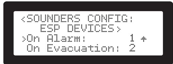
Figure 64. BUS devices configuration screen
