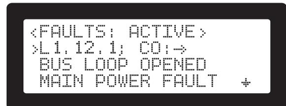
Figure 39. Fault's list screen
