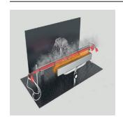
The cable is exposed for 15 minutes to flame at 650°C and for additional 15 minutes to fire and water spray.
