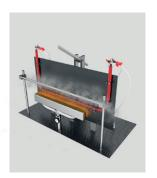
This test is carried out to verify circuit integrity during a fire. The cable is exposed to a flame at 930°C and mechanical shocks for 60 minutes and additional 60 minutes to flame, mechanical shocks and water spray..
