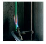
A 60 cm long sample of cable is vertically fixed with two clamps inside a small cabin, open on the front. The cable is subjected to the action of a flame produced by a calibrated Bunsen burner. The application time of the flame is according to the cable diameter (60-480 seconds). At the end of the test the burnt portion of cable must not be 50 mm close to the higher clamp.
