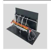
The cable is exposed to fire at the 950°C for 180 minutes.
