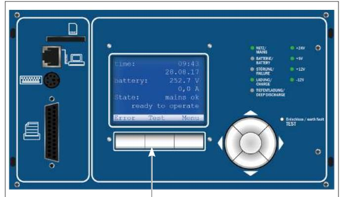
Three quick keys directly below the display are alternately used for the main commands.
